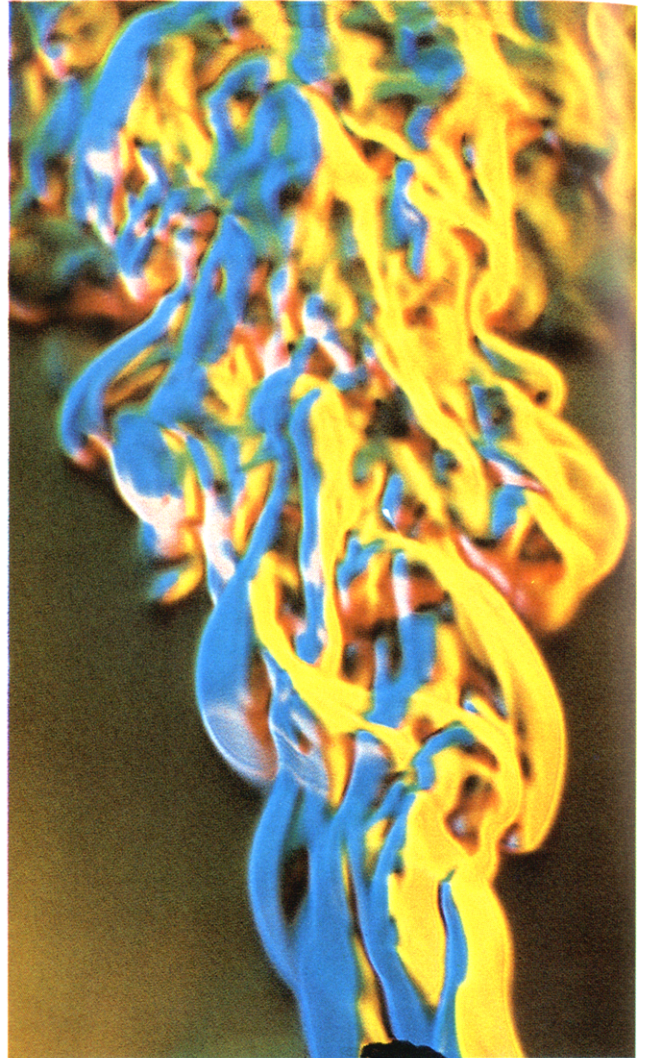
Plate 7 Turbulent flame and convection column
